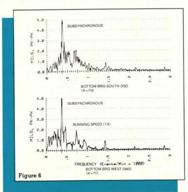
near the motor were unable to monitor the motion at the impeller. The subsynchronous activity on the impeller was not measurable at the coupling.
