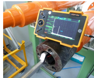
The HW-Flex probe when inspecting a hollow axle using a USM Go instrument.
