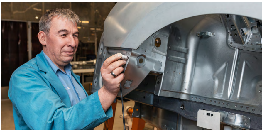
Krautkrämer SpotVision is a practical and easy-to-handle probe
