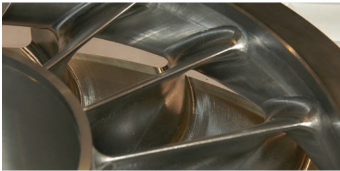
New impellers for high-mach, high-capacity compressors
