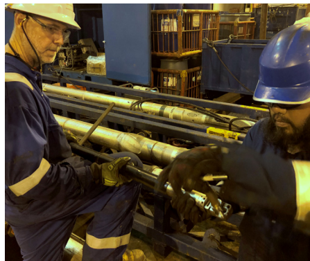
Baker Hughes engineers prepare the FASTrak HD service sample tanks.
