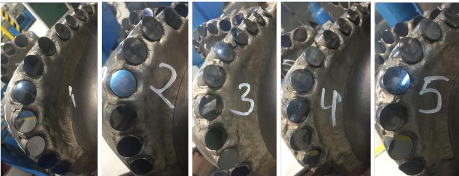
The Talon Strike PDC drill bit's cutting structure is in near-pristine condition after setting field ROP record.
