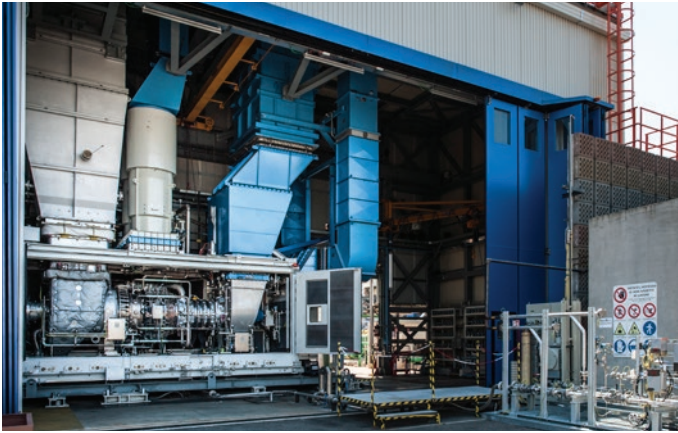
Baker Hughes NovalT™12 turbine at test bench in Florence, Italy, during hydrogen testing for Snam's Istrana project
