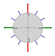
The Polar Plot assists the user in designing an optimal open hole well trajectory and open-hole completions by plotting the effects of drilling directions on critical drawdown, critical bottomhole flowing pressure and load factor.
