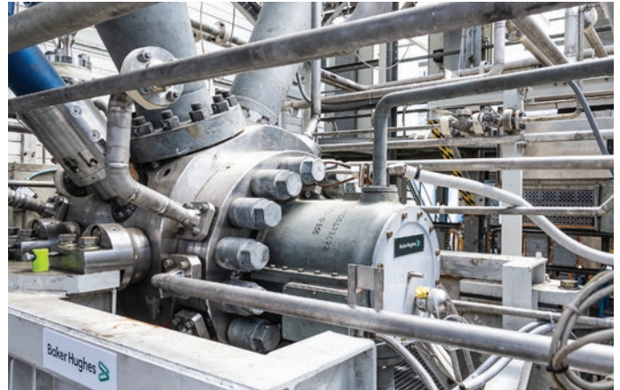
Compressor prototype installed on the test rig at the Baker Hughes facility in Florence, Italy
