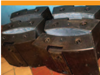
Figure 1: Examples of metallic (up) and rubber (down) segments of various guide bearings.
