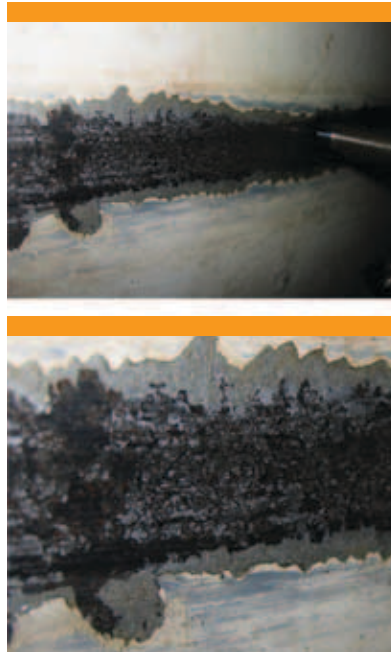
Figure 6: An example of eddy current transducer operating with a 250MW hydro-generator shaft in area close to the guide turbine bearing (upper) and closer view of the shaft surface (lower).
