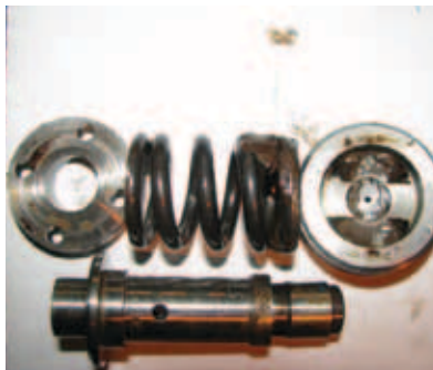
Sludge in trip bolt mechanism.
