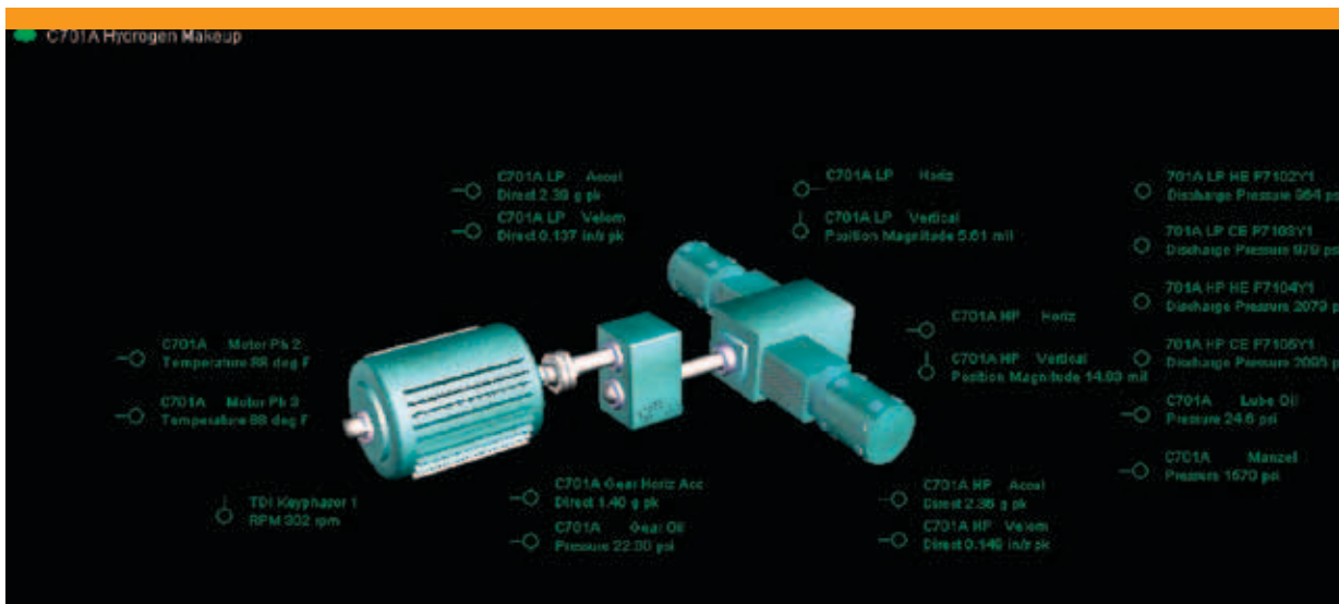
Figure 1: System 1* View of the machine train: motor, gearbox, reciprocating compressor, and parameters.
