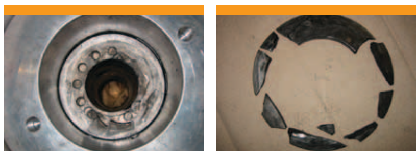
Figure 4: Minovar Piston Collar Damage
