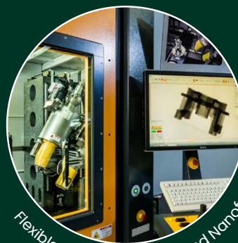
Casting CT with the powerful 300 kV Microfocus X-ray tube
