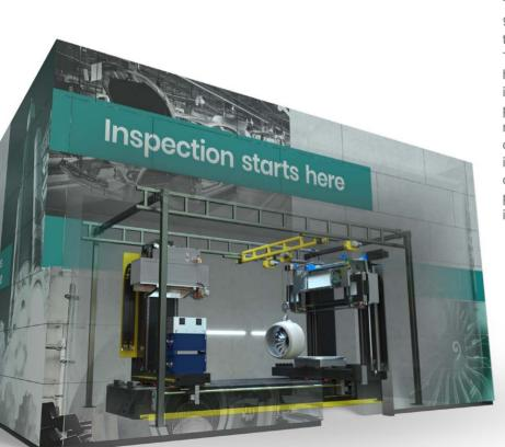
The Phoenix Power|scan HE leverages 9 MeV high-energy CT scanning technology combined with Waygate Technologies' advanced features to handle extremely large (up to 1920 mm in diameter) and heavy (up to 1000kg) parts. This system is ideal for industries requiring precision and speed, such as aerospace and automotive. It excels in scanning high-absorbing complex assemblies with unmatched efficiency, providing faster and more accurate inspections than ever before.
