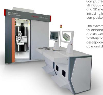
The Phoenix V|tome|x C450 is a high-performance, compact industrial CT system featuring a 450kV Minifocus X-ray tube. It is designed for the inspection and 3D metrology of a broad range of applications, including large light metal castings, turbine blades, composites, and additive manufacturing parts.
